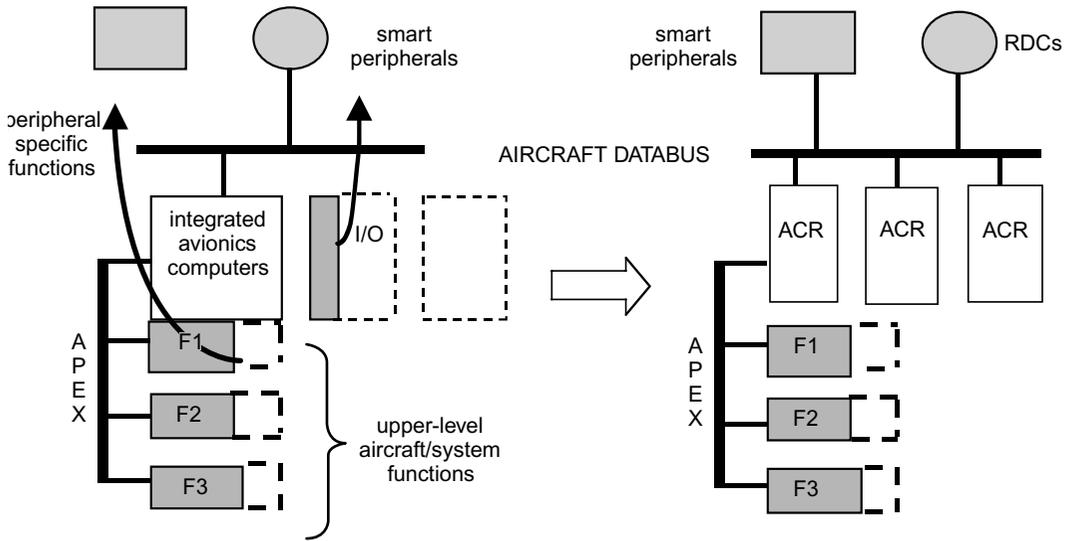
FIGURE 33.5 RDCs reduce need for analogue and discrete I/O modules.
