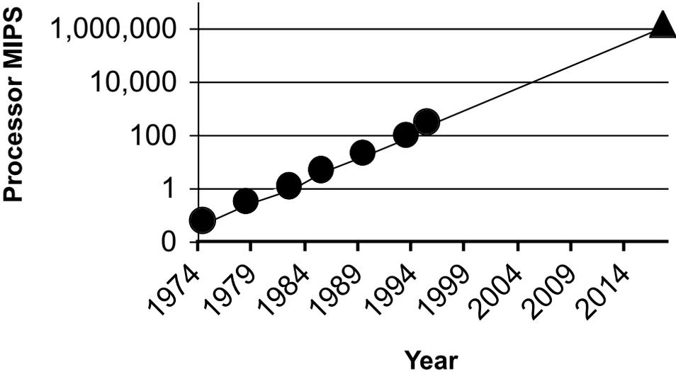
FIGURE 33.1 Increase in microprocessor performance.
